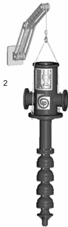
Figure 1: VIC lifted from horizontal to vertical (for pumps up to 15 feet [4.6 meters] in length)
