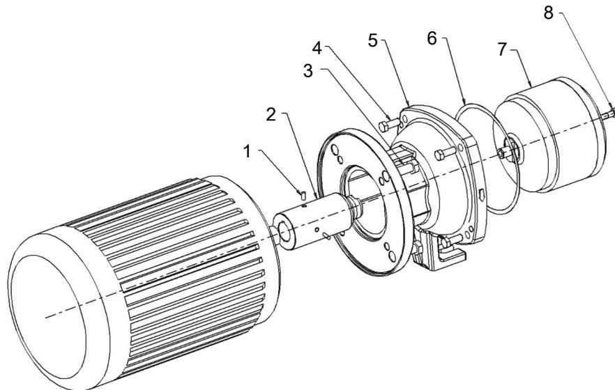
1. Stub shaft-to-motor setscrew (222L)
