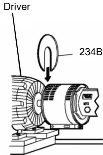
5. Remove the driver half of the coupling guard:
