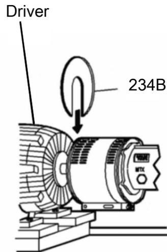
7. Place the driver-side end plate in the annular groove of the driver-half of the coupling guard.
