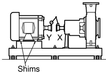
**Figure 8: Side view of an incorrect vertical alignment**
