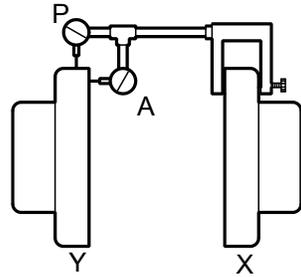
2. Rotate the pump coupling half (X) in order to check that the indicators are in contact with the driver coupling half (Y) but do not bottom out.
