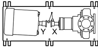
**Figure 7: Top view of an incorrect horizontal alignment**
