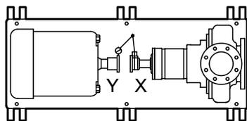
**Figure 9: Top view of an incorrect horizontal alignment**
