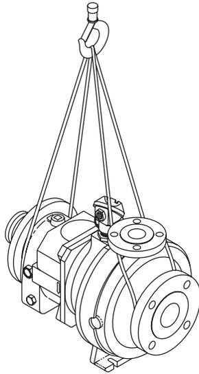
**Figure 1: Proper lifting method for a bare pump**
