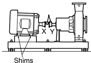
**Figure 6: Side view of an incorrect vertical alignment**
