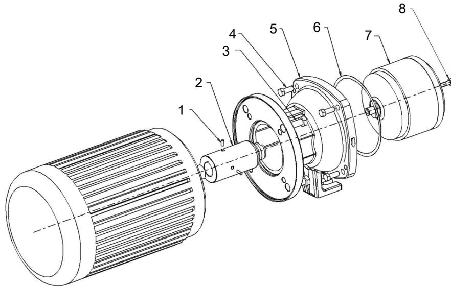
1. Stub shaft-to-motor setscrew (222L)
