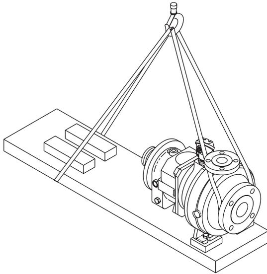
**Figure 3: Proper lifting method for a pump with a base and no driver**
