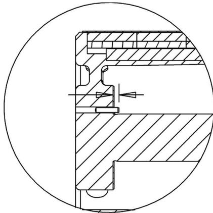
4. Cut out a small notch on the inside diameter of the intermediate ring gasket (351X) in order to create a recess for the driven carrier pin (445A) or key, depending on size.
