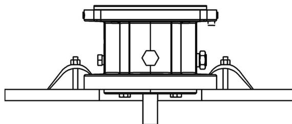
9. Mount the drive magnet assembly (740B) onto the drive shaft so that the driver cams engage. Secure the drive magnet assembly using the lockwasher (382) and capscrew (791D).
