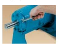
Original performance can be re-set in a matter of minutes with external impeller adjustment. Adjustable cartridge style bearing housing allows adjustment of impeller to wearplate clearance. No shims are required. No need to disassemble or drain pump.
