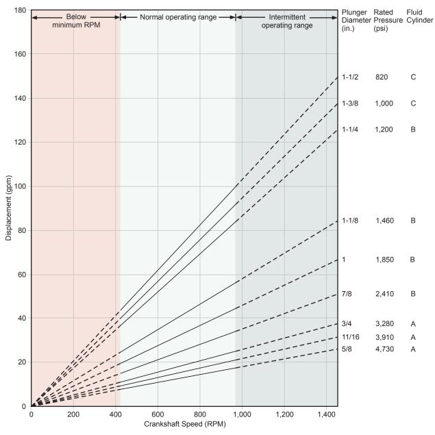
1.38-in. stroke, maximum rod load 1,450 lb (658 kg)
