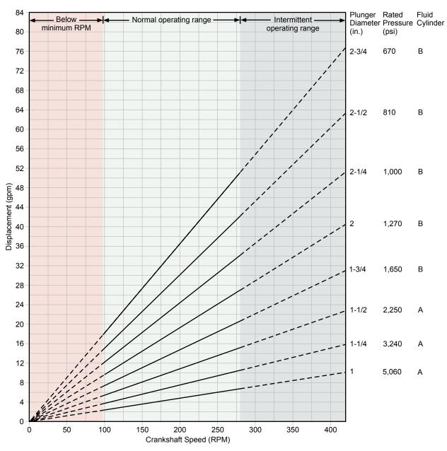
2.95-in. stroke, maximum rod load 5,500 lb (2,495 kg)
