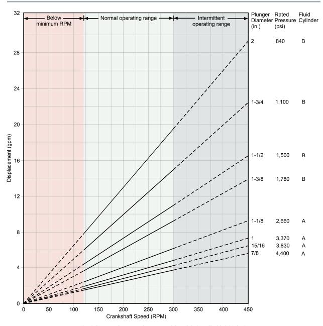
1.58-in. stroke, maximum rod load 2,645 lb (1,200 kg)
